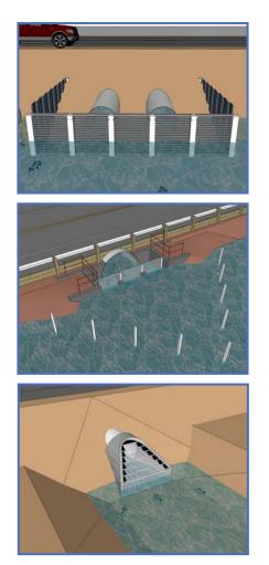
**Concept- Typo Lake outlet and North Inlet of Martin Lake**. Horizontal screens which are removable. Top of the screens serve as an emergency overflow. A maintenance catwalk and railing (not shown) will be included.
