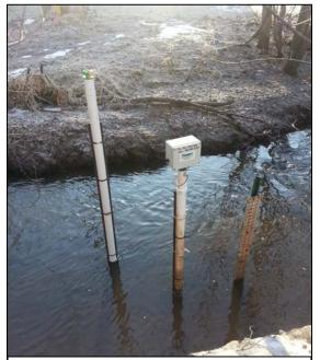
Hydrolab MS5 casing (taller) and a Measura continuous water level monitoring device I Springbrook Creek.
