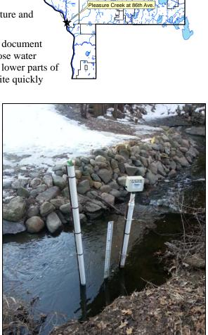
Hydrolab MS5 casing (taller) and a Measura continuous water level monitoring device in Pleasure Creek. A staff gauge is shown in the middle.
