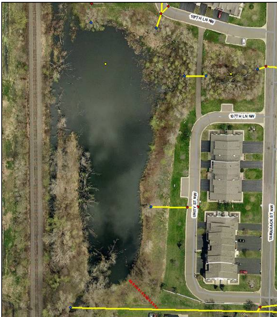
Potential re-direction of storm sewer (in red) to the Autumn Knolls pond
