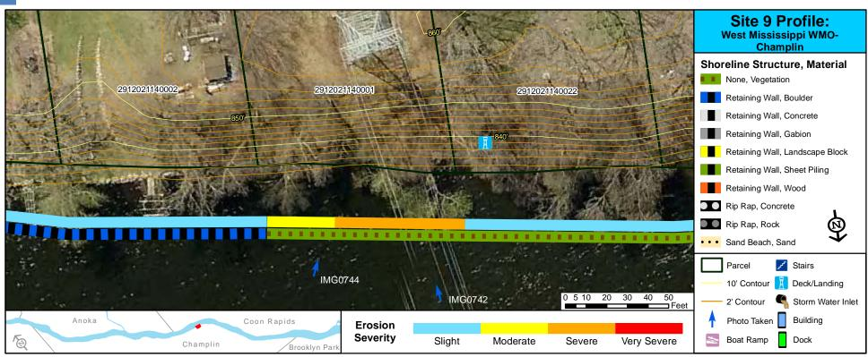
**Additional Info:** The erosion here is located directly below a transmission line. Repeated cutting of trees below the line might be contributing to the erosion here. The base of the tower is approximately 15 feet back from the top of the steep bank.
