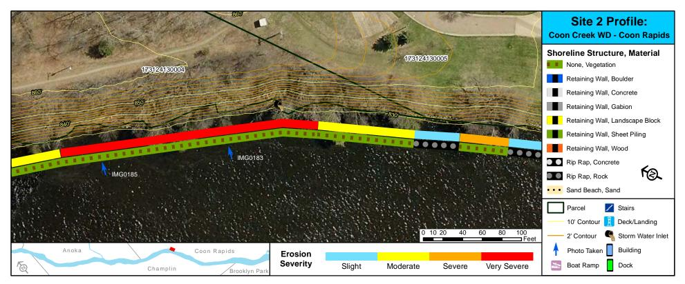
**Additional Info:** This site is located on the outside of a curve in the river, called a cut-bank. It is likely hit by large ice sheets and moving water during the spring melt. As shown in picture 183, a concrete storm water culvert is sticking 5 feet out from the sheer bank. This along with the many slumping trees at the site show the large amount of sediment lost.
