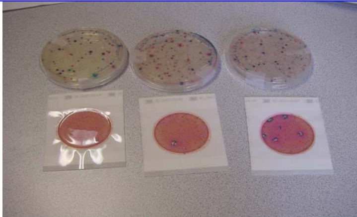
Two kinds of do-it-yourself test kits used to quantify E. coli in Pleasure Creek. A certified laboratory provides a third method
