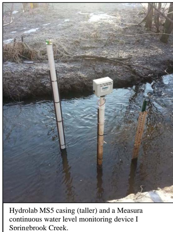
Hydrolab MS5 casing (taller) and a Measura continuous water level monitoring device I Springbrook Creek.
