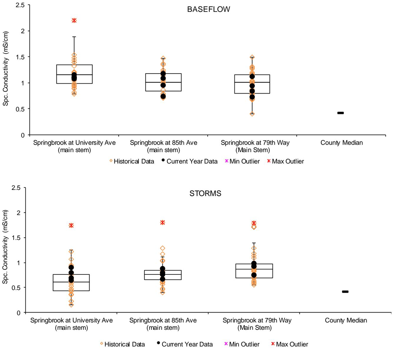
**Chlorides at Springbrook Creek.** Orange diamonds are historical data from previous years and black circles are 2019 readings. Box plots show the median (middle line), 25<sup>th</sup> and 75<sup>th</sup> percentile (ends of box), and 10<sup>th</sup> and 90<sup>th</sup> percentiles (floating outer lines).
