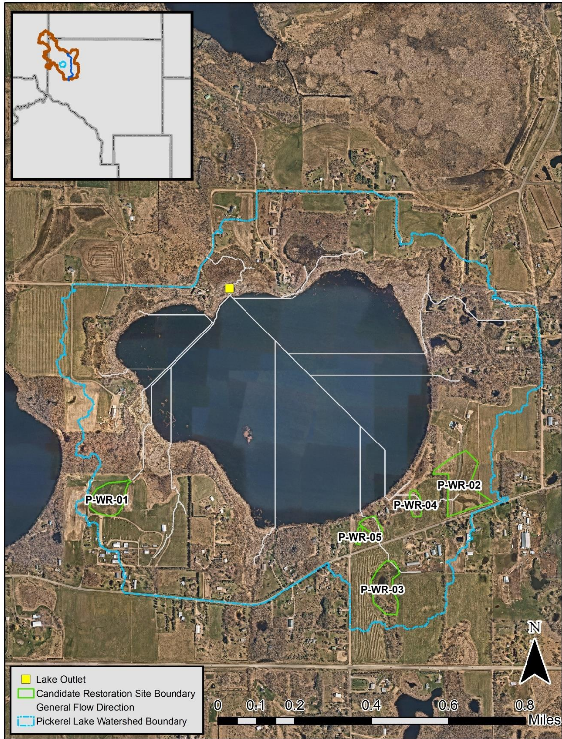
Figure 11. Candidate wetland restoration locations in the Pickrel Lake subwatershed. See Table 5 for a summary of each project's estimated benefits.
