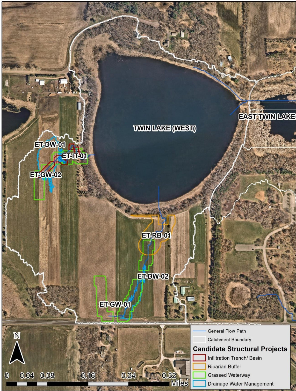
Figure 10. Candidate structural projects sited in the East Twin Lake watershed. Source reduction practices were also generated here and could be applied to the entire cropped field. See details for each project in Table 3.
