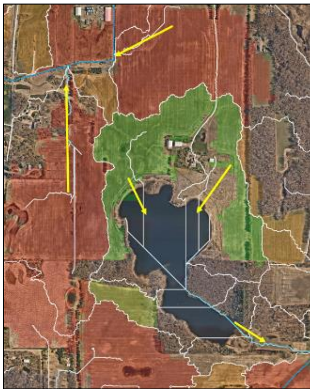
Figure 12. Catchment boundaries and flow paths for a cultivated field adjacent to Ford Brook. Portions of the field draining directly to ditch networks contribute the greatest pollutant loads to Ford Brook through these direct hydrologic connections, whereas runoff passing through other features, such as this shallow lake, likely loses much of its pollutant load prior to entering the Ford Brook channel.
